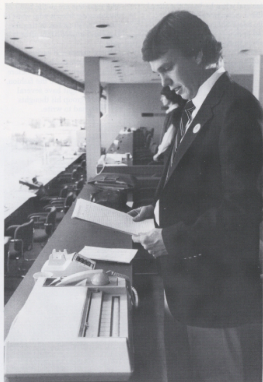
Telecopiers were used to send stories back to the press before the advent of video display terminals.
